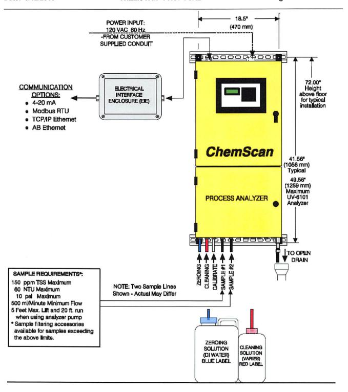
ChemScan Process Analyzer -Typical Installation Diagram
