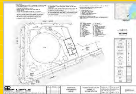
Exhibit 3-7 / Brown & Phillips performed topographic surveys of two repump stations at Avenue C and Avenue U for the RBUD for the design of improvements.
