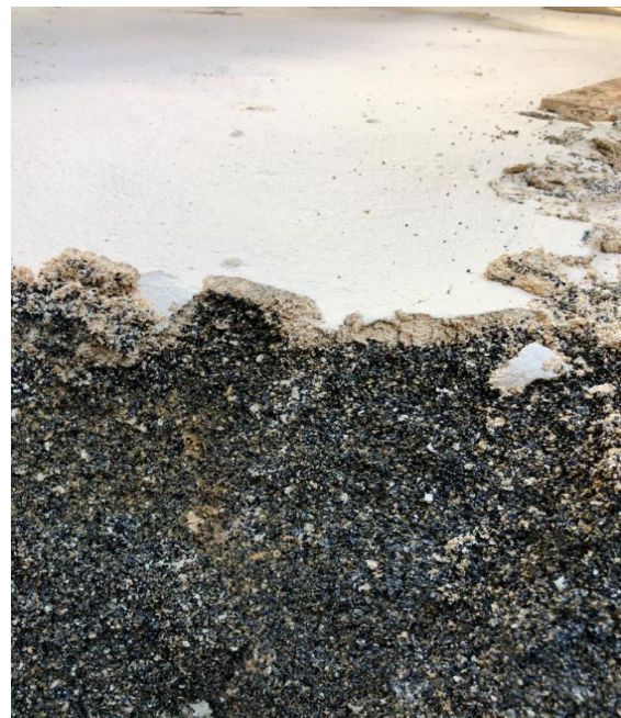
Figure 4-6. Cross-section of Washed Filter Bed
