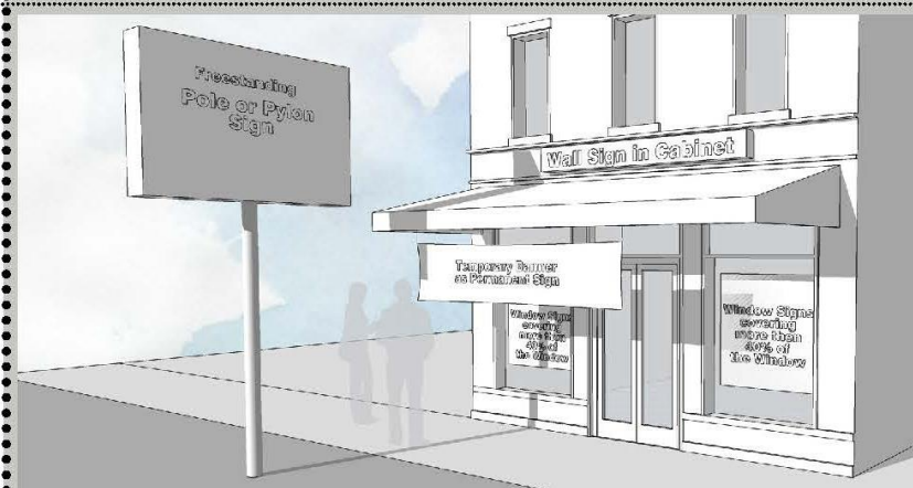
Figure 61 Activity inside is obscured by banners and window coverings. The materials such as plastic face-lit cabinets and banners are not durable and long lasting. The pole sign is too high and contributes to signage clutter and does not address the pedestrian.
