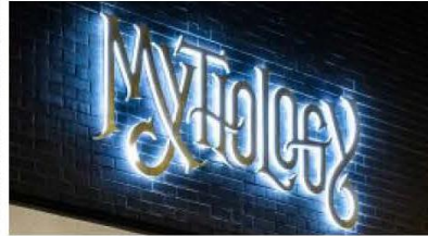
Figure 55 Reverse channel LED halo-lit letters
