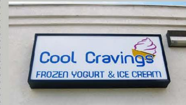
Figure 47 Face illuminated cabinet sign
