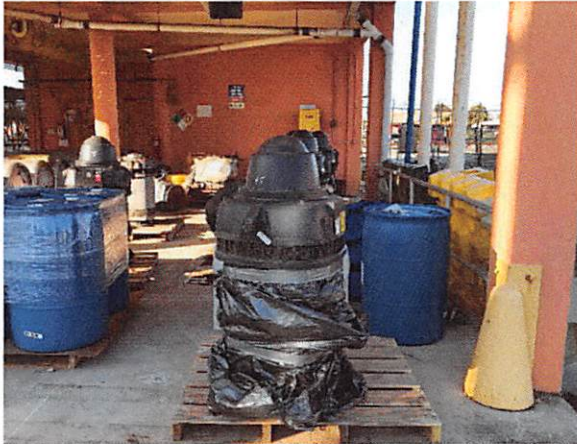
Figure 10. New uninstalled HSP motors
