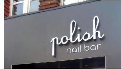
Figure 56 Front-lit LED channel letters with translucent acrylic faces
