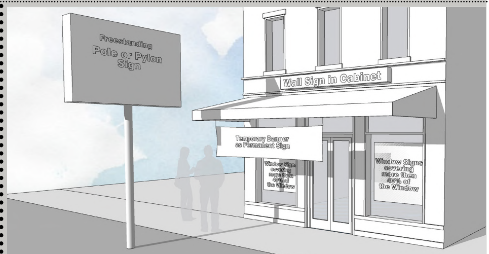
Figure 61 Activity inside is obscured by banners and window coverings. The materials such as plastic face-lit cabinets and banners are not durable and long lasting. The pole sign is too high and contributes to signage clutter and does not address the pedestrian.
