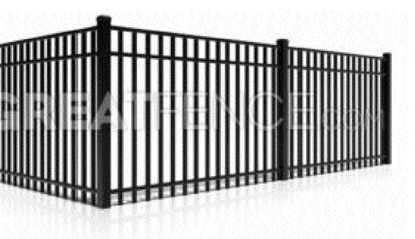
5' FENCE: BY GREATFENCE.COM. COMMERCIAL STYLE 4 OR APPROVED EQUAL. FENCE SHALL BE 5'-0" HEIGHT ALUMINUM PICKET FENCE WITH FLAT TOP RAIL AND BOTTOM RAIL; PICKET SPACING AND SIZES SHALL BE AS PER APPLICABLE CODE REQUIREMENTS. ALL PEDESTRIAN EGRESS AND INGRESS GATES SHALL BE SELF-LOCKING WITH A SELF -LATCHING MECHANISM AND COMPLY WITH APPLICABLE CODE REQUIREMENTS.
