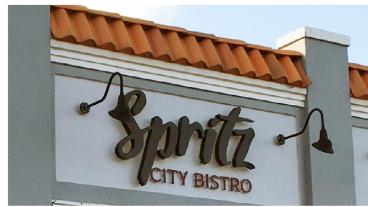
Figure 3 Reverse illuminated channel letters on concealed raceway
