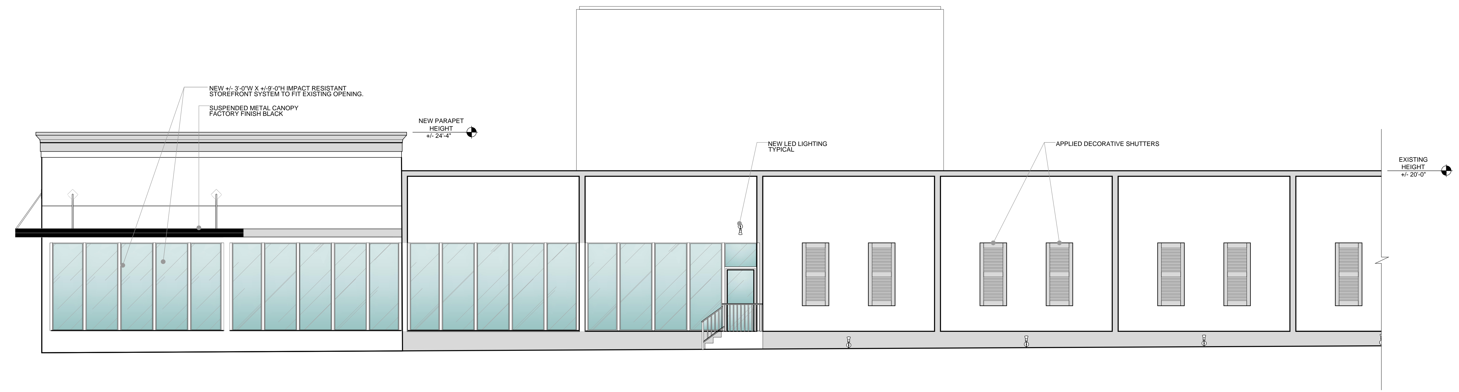
ENLARGED NORTH - EAST END ELEVATION 2 FOAM TRIM CORNICE WITH ACRYLIC FINISH TO MATCH STUCCO. PROFILE TO MATCH EXISTING. SCALE: 3/16" = 1'-0"
