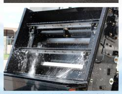
HEAVY SWEEP PACKAGE Elevator Type: Standard 11 Flight squeegee with replaceable corded rubber tips; Continuous molded rubber belts combined with standard Heavy Sweep Package make Global M4 the logical choice for sweeping heavy debris such as road millings, sand and gravel up to 3-Tons per-Minute. That is one ton of sand every 20 seconds! Standard leaf gate system assists in picking up large debris, bottles, large branches and leaves.
