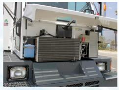
ACCESS IT ALL The Global M4 features many maintenance-friendly attributes, such as a rear swing-out radiator, easy access front mounted AC condenser, brake and windshield washer fluid reservoirs, and cab fresh air filter.
