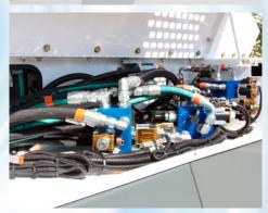
IT'S ALL IN THE OPEN Hydraulic Hoses are NOT hidden in the frame of the sweeper, while all Manifolds and Filters are located in a central location.
