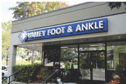
FACE & REVERSE ILLUMINATED CHANNEL LETTERS MOUNTED ON WIREWAY
