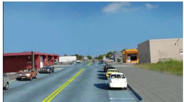
Phase 1: To enhance retail and calm traffic, on-street parking, curb, gutter, and sidewalks are added.
